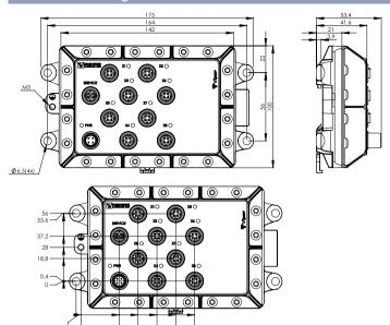
Weight 0.9 kg Degree of protection IP65
