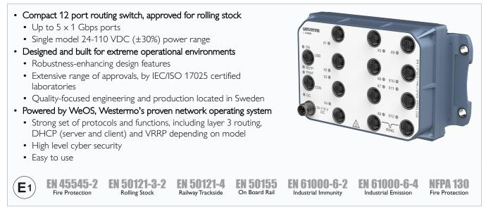
The Viper-12A series consists of managed 12 port routing switches optimised for the needs of the railway rolling stock market. Gbps ports cope with high bandwidth devices such as access points and NVRs (Network Video Recorders).
