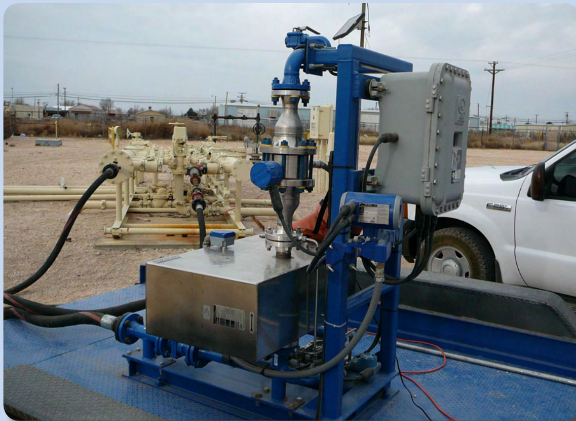
Typical 2" MPFM-50. Trailer Mounted Version
